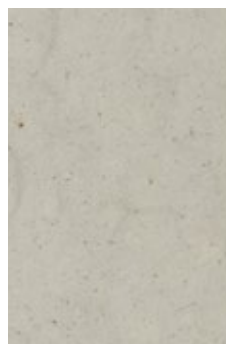
普通彩板挂片半年后的 实物 Actual view of common prepainted steel sheets applied after half a year
