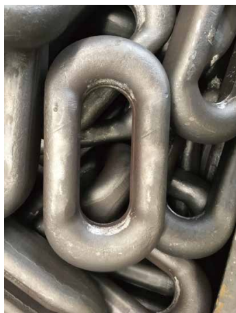
23MnNiMoCr54 圆环 (用户提供) Round link chains of 23MnNiMoCr54 (Photo courtesy of a customer)
