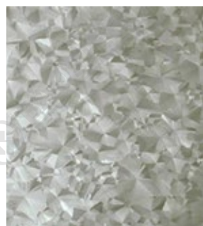
正常（不平整）锌花 Normal (non-skinpassed) spangle
