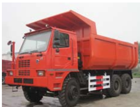
采用宝钢热轧耐磨钢BW450制造的矿用重型自卸车 Tipper body of heavy dump truck using hot rolled BW450 of Baosteel
