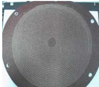
图2 测试后砂纸表面的螺旋线 FIG. 2 spiral line on the coated abrasive disk after test
