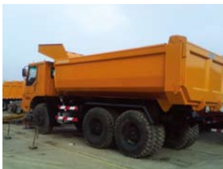
采用宝钢热轧耐磨钢BW400制造的矿用重型自卸车 Tipper body of heavy dump truck using hot rolled BW400 of Baosteel
