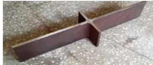
十字接头 (Cruciform joint)
