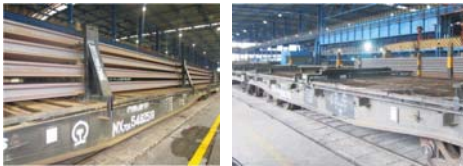
100米钢轨专用转向架 Special bogie for 100-meter rail
