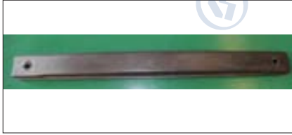
Hot stamped front bumper (B1800HS, thickness of 1.2 mm)
