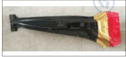
Hot-stamped B-pillar with variable strength (B1500HS, thickness of 1.2 mm)
