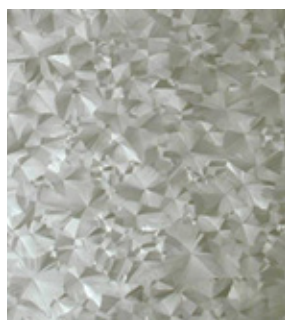
正常 (不平整) 锌花 Normal (non-skinpassed) spangle
