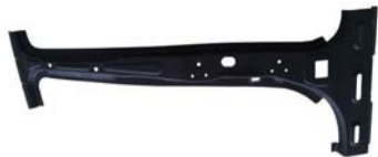
图20 热冲压B柱, B1500HS, 1.8mm × 1025mm
