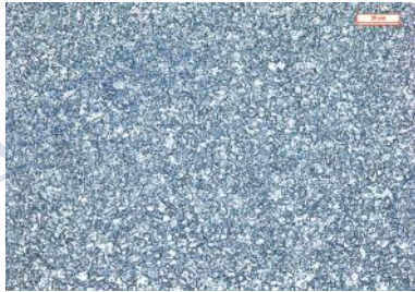
Fig.11 Typical microstructure of cold rolled CP steel
