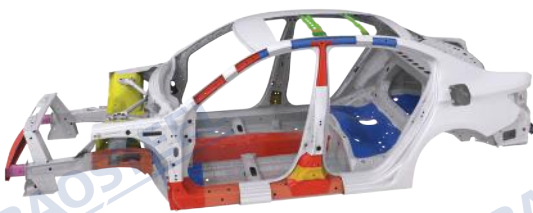
Fig.2 Main applications of AHSS for auto body (Baosteel Car Body)
