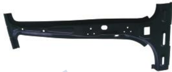
Fig.20 B-pillar, HC950/1300HS (1.8mm×1025mm)
