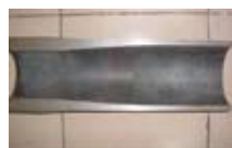
长且平滑的内加厚过渡区 Long and smooth taper of internal upset
