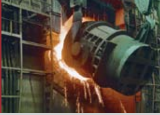
300 吨氧气顶底复吹转炉 300t combined top and bottom oxygen blowing converter
